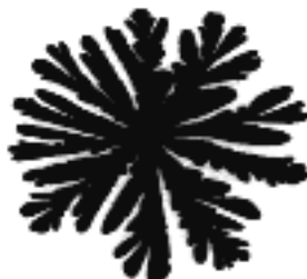
Figure 4.11: Hele-Shaw experiments showing the less viscous colored water injected into the more viscous glycerin.
