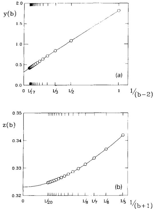
Fig. 2. (a) Quantity  $y(b)$  defined by eq. (10a) versus  $1/(b-2)$ . The solid straight line represents the best fit of the exact data (obtained for  $b \approx 19$ ) using the variable  $1/(b-2)$ . (b) Quantity  $z(b)$  defined by (10b) versus  $1/(b+1)$ . The solid curve represents the best fit of the exact data to a third order polynomial in  $1/(b+1)$ .
