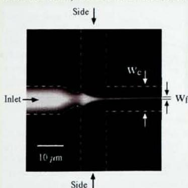
second. At this rate a shot of espresso would take a year to deliver. The Princeton mixer, frugal with expensive samples and compact enough to sit on a silicon chip, makes it possible to study fast reaction kinetics at previously unattainable time scales. For example, proteins fold in response to quick changes in concentration of the "denaturant" in the solvent surrounding them. (J. B. Knight *et al.*, *Phys. Rev. Lett.* **80**, 3863, 1998.) —PFS
