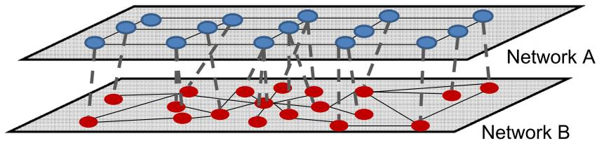
**Fig. 1.** Example of two interdependent networks. Nodes in network B (communications network) are dependent on nodes in network A (power grid) for power; nodes in network A are dependent on network B for control information.
