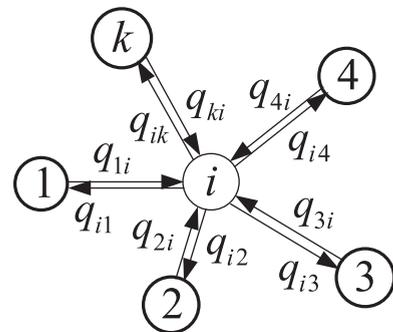
**Fig. 7.** Schematic representation of a network of networks. Circles represent interdependent networks, and the arrows connect the partially interdependent pairs. For example, a fraction of  $q_{3i}$  of nodes in network  $i$  depend on the nodes in network 3. The networks which are not connected by the dependency links do not have nodes that directly depend on one another. After Gao et al. [49].
