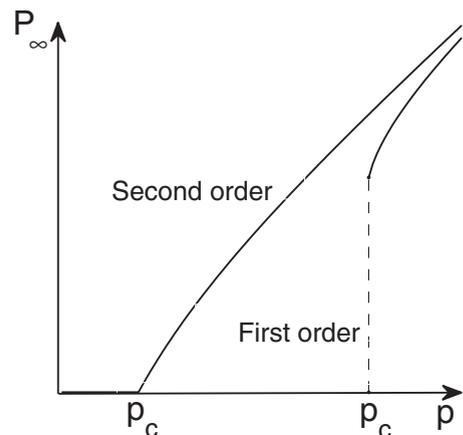
**Fig. 2.** Schematic demonstration of first and second order percolation transitions. In the second order case, the giant component is continuously approaching zero at the percolation threshold  $p = p_c$ . In the first order case the giant component approaches zero discontinuously. After Gao et al. [49].
