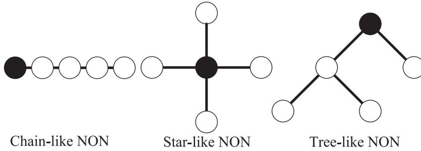
**Fig. 8.** Three types of loopless networks of networks composed of five coupled networks. All have same percolation threshold and same giant component. The dark node is the origin network on which failures initially occur. After Gao et al. [49].
