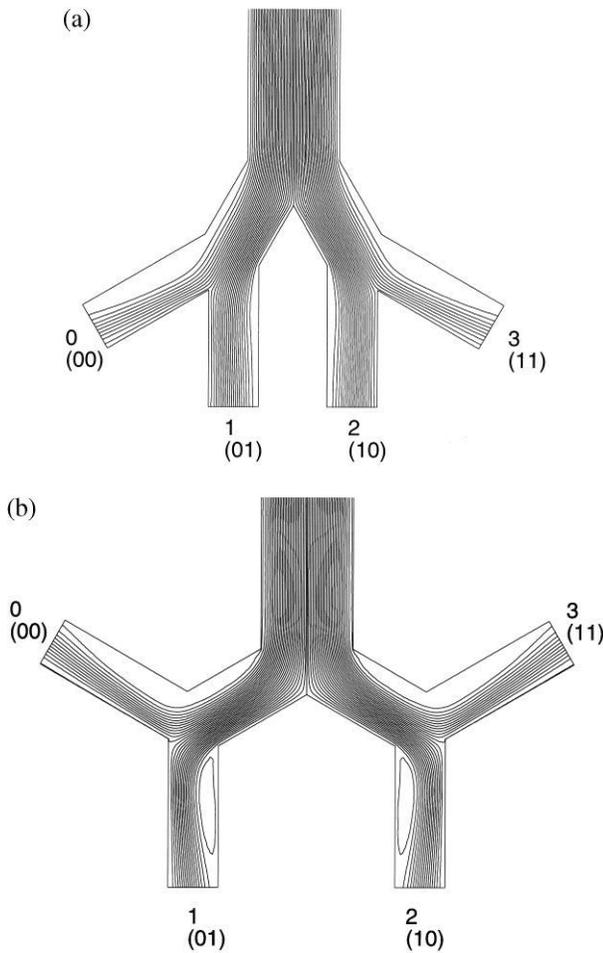
FIG. 3. (a) Contour plot of the stream function in a three-generation tree with branching angle  $\theta = 30^\circ$  and  $Re = 1200$ . (b) Same as in (a) but for  $\theta = 60^\circ$ . Note that the number of streamlines and thus the fluxes at outlets 1 and 2 are larger in (a) than in (b). Also shown is the binary representation of each outlet branch.
