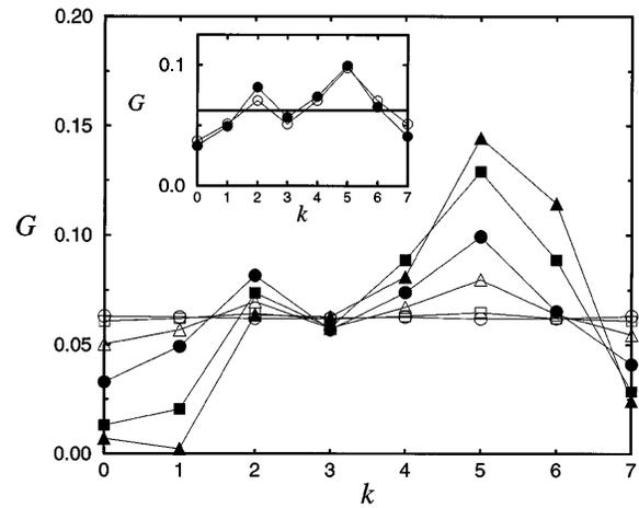
FIG. 2. Flux distribution at the outlet branches of a five-generation tree for  $Re = 150$  (circle), 300 (square), 600 (triangle), 1200 (full circle), 2400 (full square), and 4800 (full triangle). The inset compares the fluid flow simulations ( $Re = 1200$ , circle) and the binary tree model ( $p = 0.58$ , full circle).
