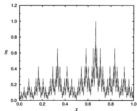
FIG. 5. Distribution of normalized fluxes  $g(x)$  defined in Eq. (2) as a function of the normalized branch number  $x$  at the outlets of an 11-generation tree with a partitioning factor  $p = 0.6$ , calculated using the binary tree model.
